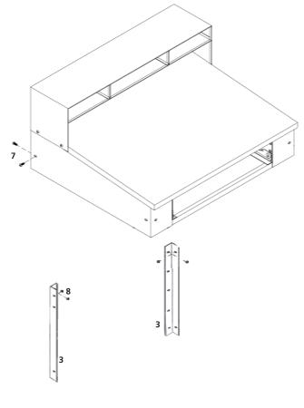
**3.** Attach the front angled legs (Ref. No. 4) to the front of the unit, using four nuts and bolts on each leg. Next, attach the front legs to the rear legs, using a nut and bolt on each side.
